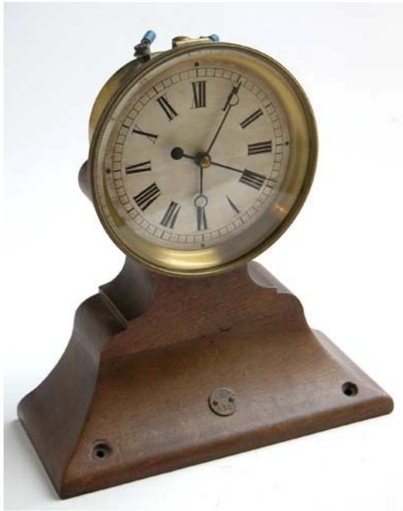
Favarger bench-clock for seconds-impulses, case
