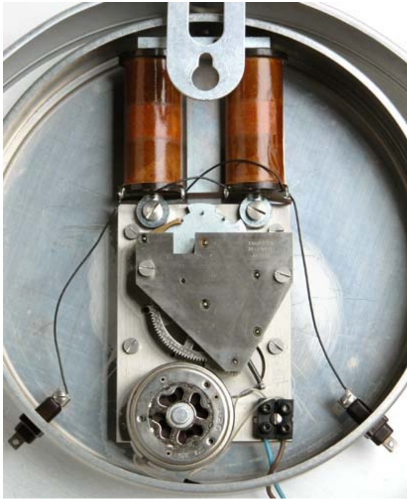
Favag with synchronous motor for the seconds (Swiss railway)
